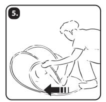
Push the cross-over away from you in a straight line for 40-50cm until the metal loops start to fold.
